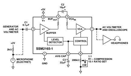
Figure 8. Electret Microphone Preamp Example
