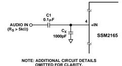
Figure 7. Circuit Configuration for Use with High Impedance Signal Sources
