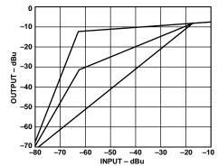
Figure 1b. SSM2165-2 Compression and Gating Characteristics
