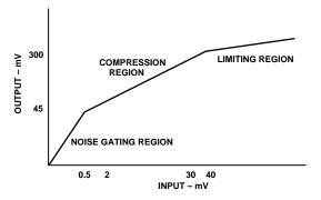
Figure 10. Transfer Characteristic
