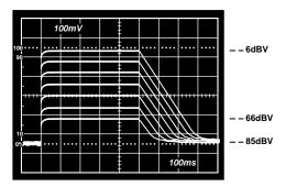
Figure 4. RMS Level Detector Performance with  $C_{AVG} = 2.2 \,\mu F$
