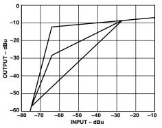
Figure 1a. SSM2165-1 Compression and Gating Characteristics
