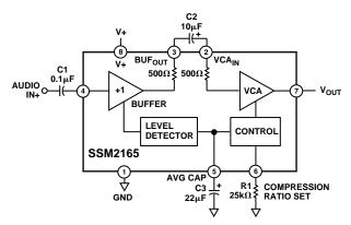
Figure 3. Functional Block Diagram and Typical Voice Application
